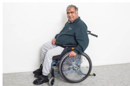
*With the rear wheels moved forward, Mannan can comfortably start the propulsion from the top of the handrim.*
