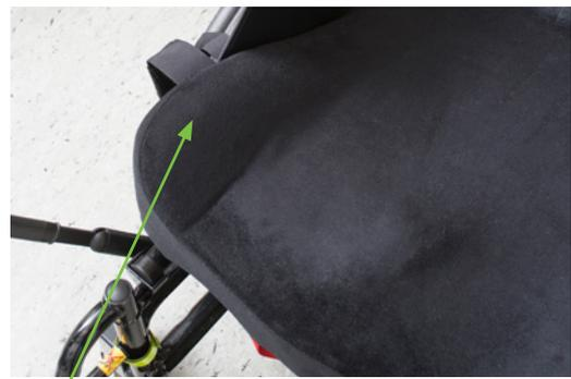
*The seat cushion has built in lateral support. The right side had insufficient support and his left side was hurting when he foot propelled.*
