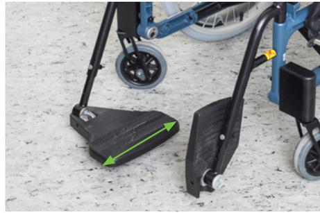
The right foot support is equipped with an extension. The wider castor housings allow more space for foot propulsion.
